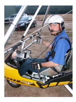
Without finger function I had developed an adaptation that connects to the control bar, allowing me to be able to lock my hands in place to steer the wing in flight.
